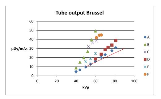
Figure 7: Overview of the tube output for Brussels. The inferior limit of acceptability of the tube output is reported (red line).
