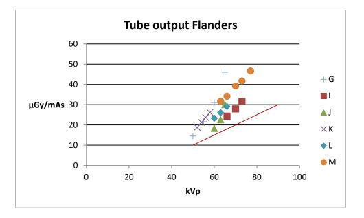
Figure 8: Overview of the tube outputs for Flanders. The inferior limit of acceptability of the tube output is reported (red line).
