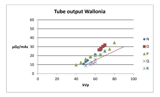
Figure 9: Overview of the tube outputs Wallonia. The inferior limit of acceptability of the tube output is reported (red line).
